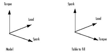
In the diagram of a table shown, the *x*- and *y*-axes represent the normalizers (which you want to be spark and load) and the *z*-axis is the output at each breakpoint (torque). To fill this table correctly from the model is a two-step process. First you need to fill a table that has the same input and output as the model, and then fill a second table by inversion.
